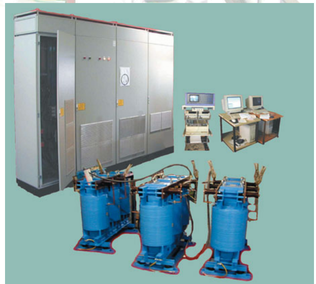
Fig. 5: Harmonic generator for real load tests
