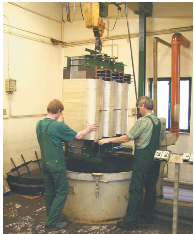
Fig. 9: Vacuum/overpressure impregnation equipment
