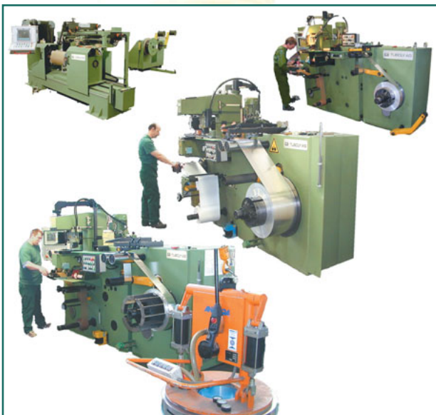
Fig. 8: Computer controlled winding machines
